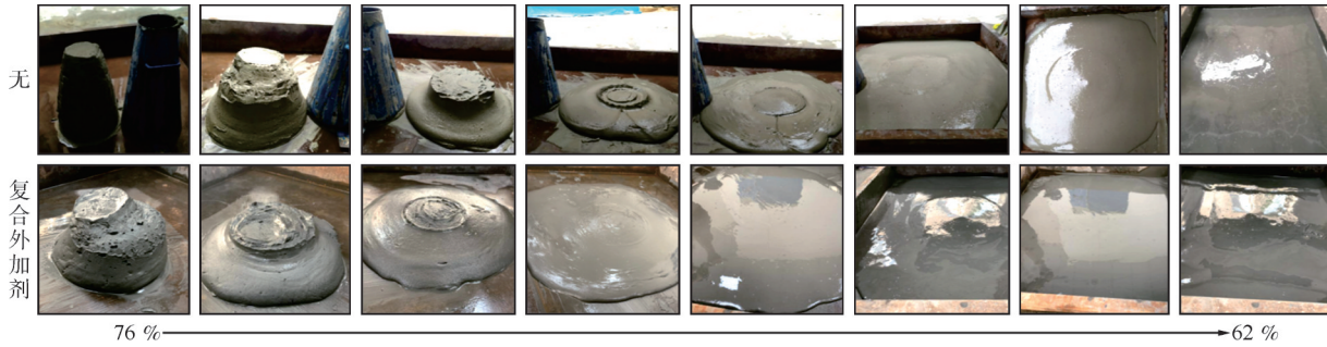
图4 含/不含复合外加剂充填料浆塌落度实拍 Fig. 4 Photos of slump of slurry with/without compound additive
